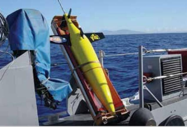
Left: SeaGlider, developed at the University of Washington, USA, is a freely roving craft that can be deployed at sea for many weeks. Undulating from the surface to depths of about 500 m it travels slowly through the ocean and transmits data back to a lab at sea or on-shore via satellites. Image: University of Washington.
