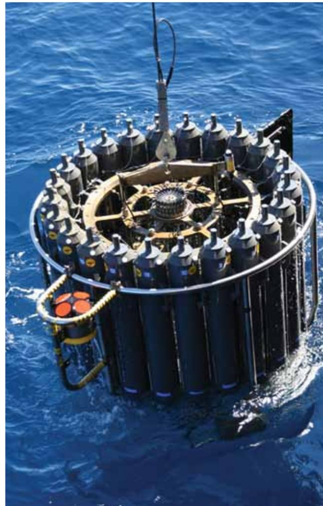
A rosette of filled (24 x 20 litre) water-sampling bottles is hoisted on-board with a steel conducting cable. The orange instrument is an upward looking Acoustic Doppler Profiler (ADCP) that measures current velocities by tracking particle movements in the water. Image: Mike Lucas
