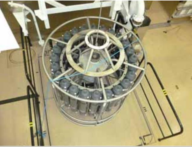
Left below: A rosette of 24 x 20 litre water-sampling bottles stands on top of the trap-door access to the 'moon pool'. The circular 'docking head' on top ensures the rosette can be carefully lowered through the hull below the ship. Image: Mike Lucas
